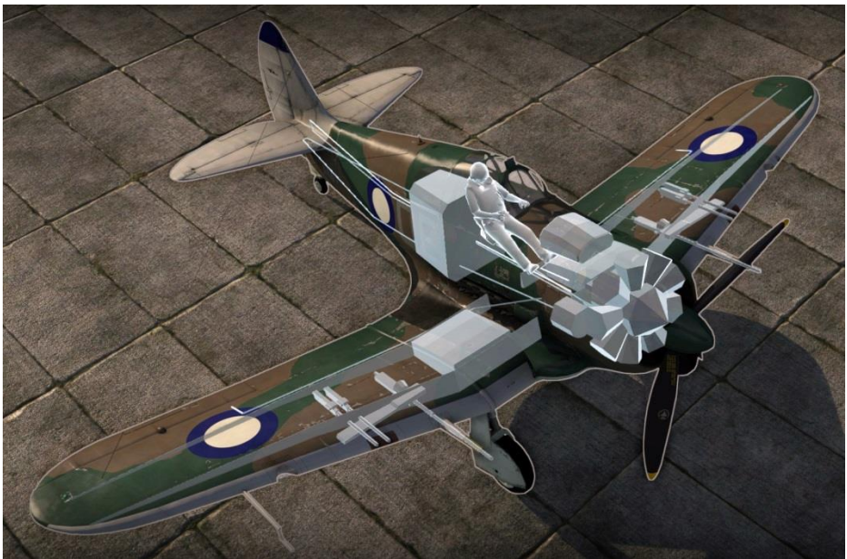
X-ray view of the RAAF Boomerang Mk.II
