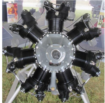
The Continental R-670 radial aircraft engine that powered the M2 - fast enough to launch itself off earth mounds
