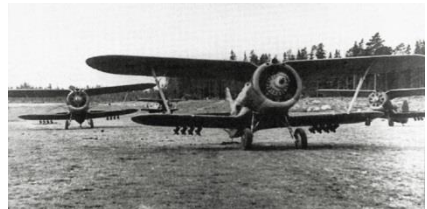
A group of I-153 equipped with ground attack rockets preparing for liftoff
